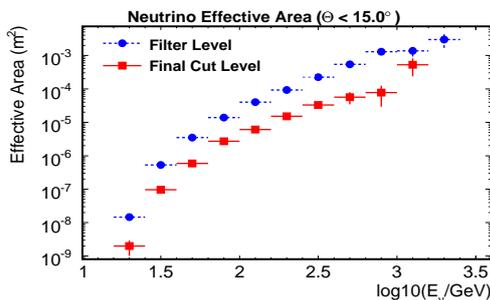
Fig. 4. Average muon neutrino effective area for vertical up-going neutrinos (within 15 degree's of vertical direction) as function of neutrino energy.
